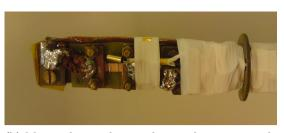
(b) Mounted sample on the single axis sample holder.
