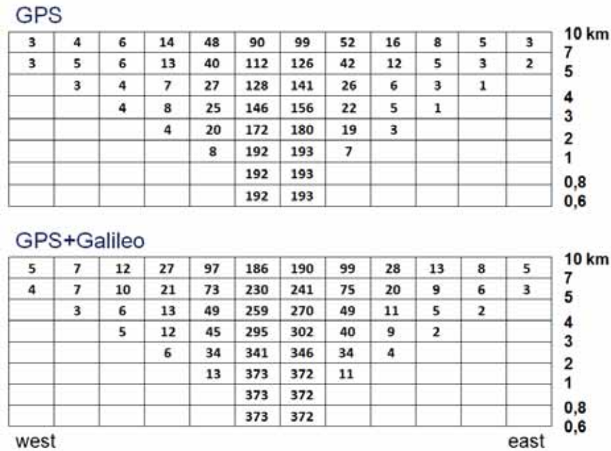
Figure 7.4: Simulated raytraced tomography model using GPS-only and GPS+Galileo observations (number of observations per voxel)
