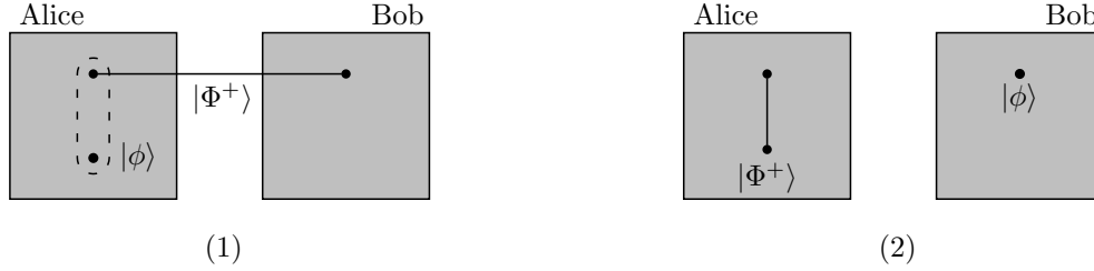
Figure 2.3: ( Teleportation ) Alice and Bob share a Bell state of the form |\Phi^+\rangle_{AB} . Here, the dashed line indicates a measurement in the Bell basis.
