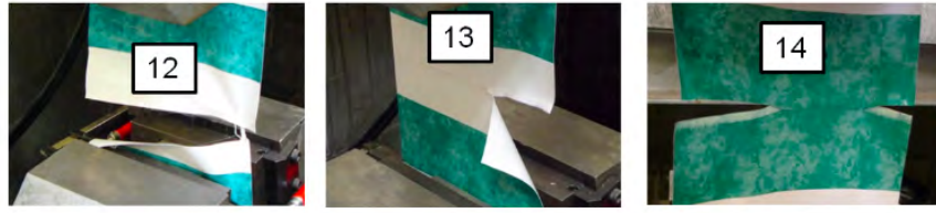
Figure 5.3: Welded seams - specimen 12 to 14
