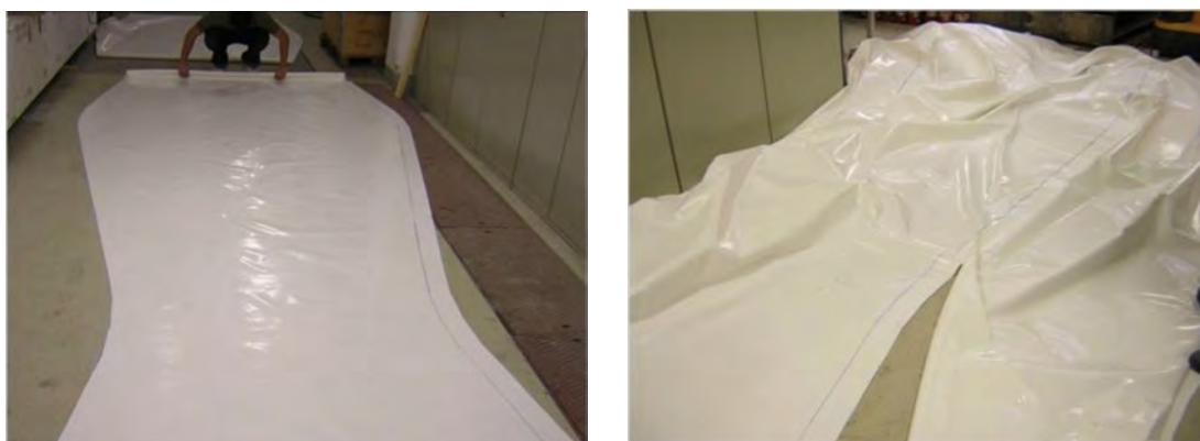
Figure 10.12: Production of the pneumatic formwork
