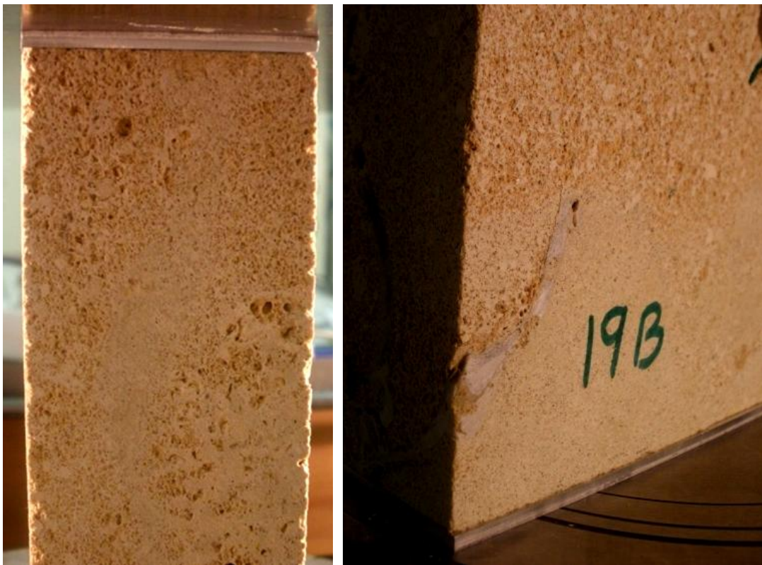
Fig. 5.24: Cracks in specimen 19 for point 1 of the figure 5.23. a) Cracks on right side of the specimen. b) Cracks on the side B of the specimen.
