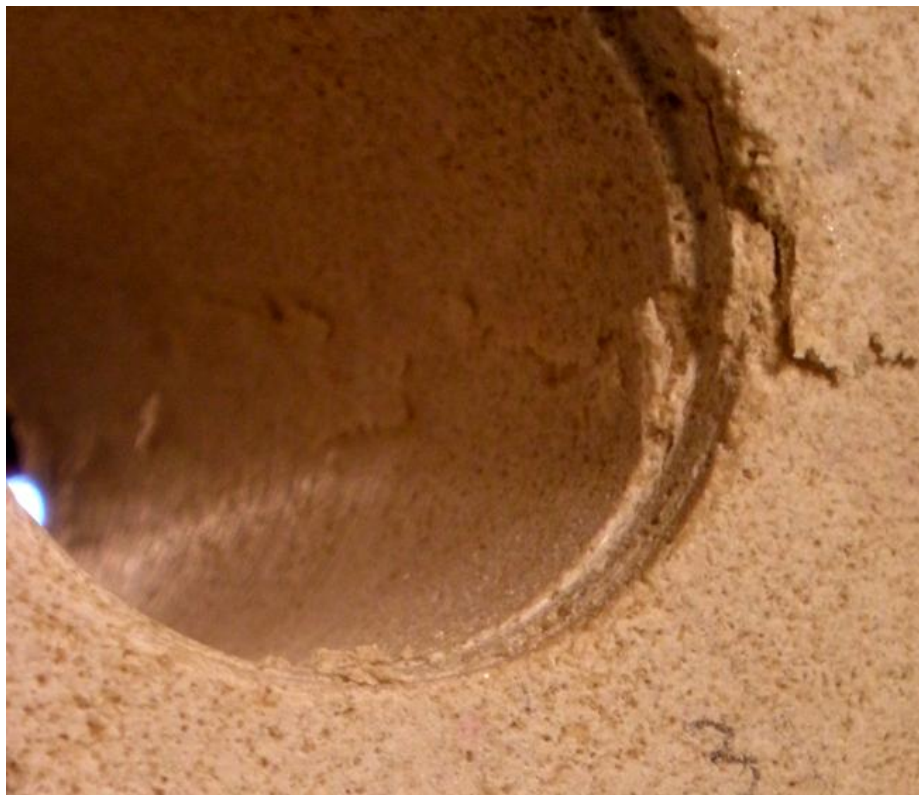
Fig. 5.41: Cracks in specimen 22 for point 2 of the figure 5.38. Rupture on the right wall of the drillhole. Picture was taken from side A of the specimen.
