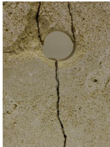
Fig.9.10: Specimen 7 after testing. a) Side A. b) Side B. c) Drillhole of the specimen. (Left) The drillhole was photographed from side A. (Right) .The drillhole was photographed from side B.
