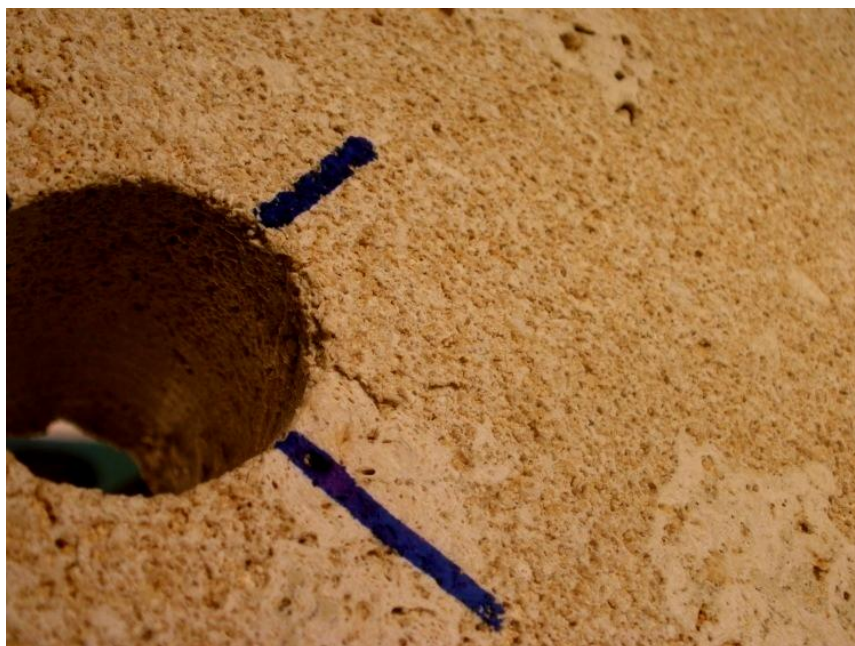
Fig. 5.33: Cracks in specimen 19 for point 9 of the figure 5.23. Cracks on the side A of the specimen.
