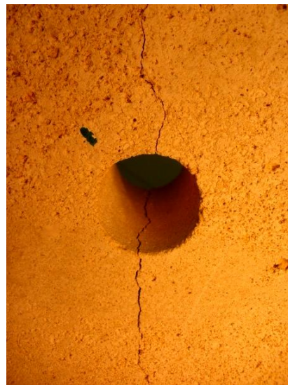
Fig. 9.9: Specimen 6 after testing. a) Side A. b) Side B. c) Drillhole of the specimen. (Left) The drillhole was photographed from side A. (Right). The drillhole was photographed from side B.
