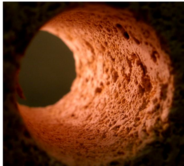
Fig.9.15: Specimen 12 after testing. a) Side A. b) Side B. c) Drillhole of the specimen. (Left) The drillhole was photographed from side A. (Right) The drillhole was photographed from side B.
