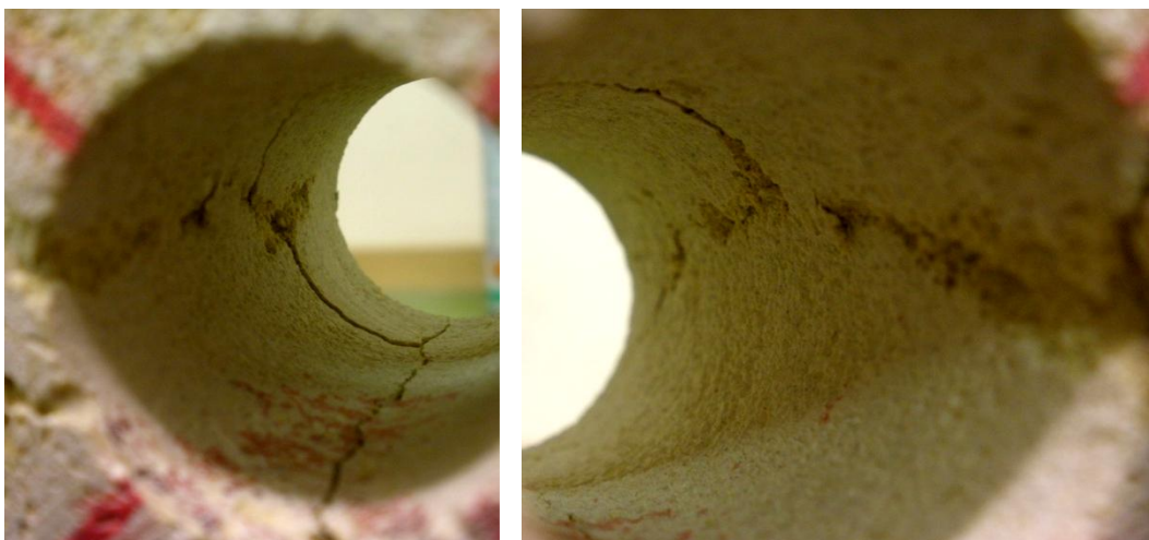
Fig. 9.5: Specimen 1 after testing 1a. a) Side A. b) Side B. c) Drillhole of the specimen. The drillhole was photographed from side A.
