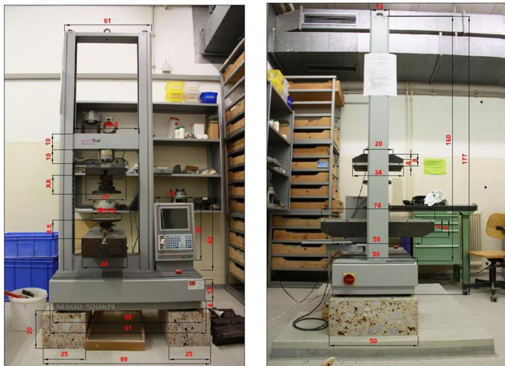
Fig. 9.28: Testing machine for compression test. Small machine.
