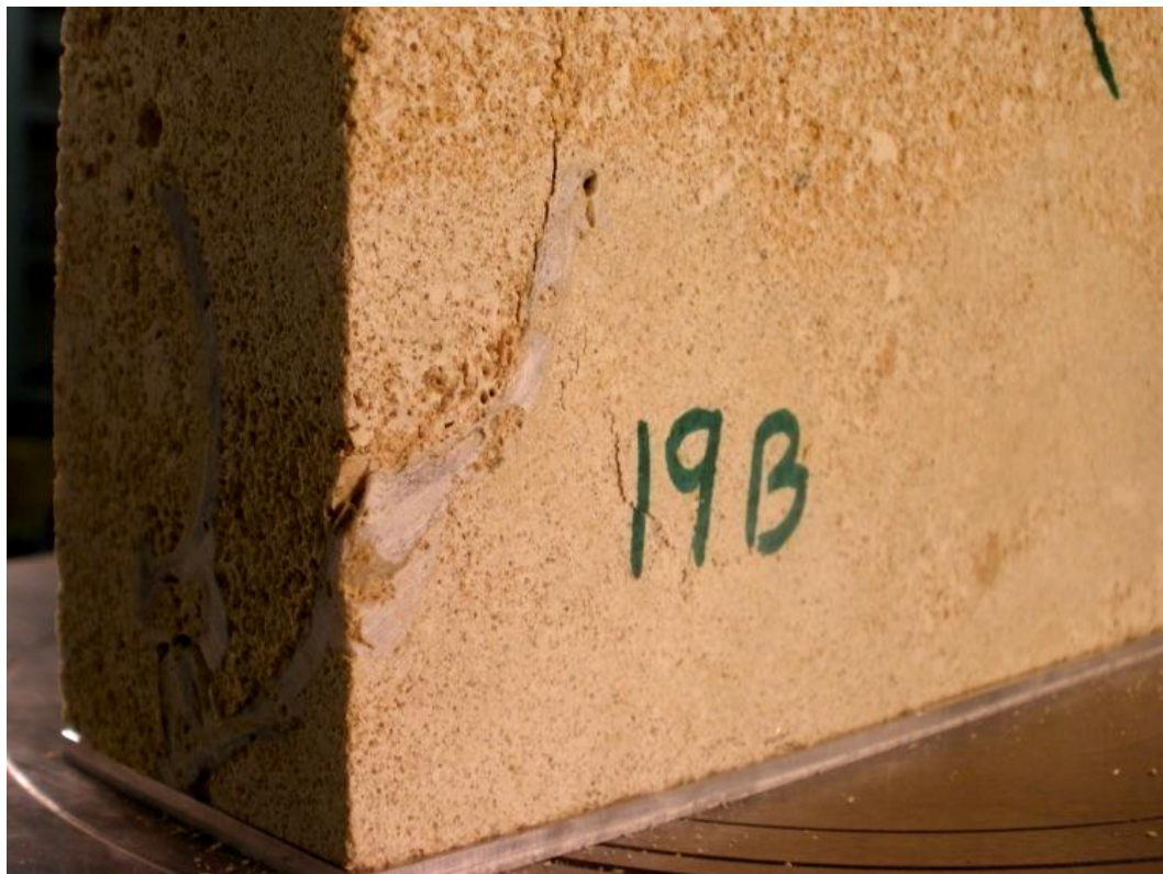
Fig. 5.28: Cracks in specimen 19 for point 5 of the figure 5.23. Cracks on the side B of the specimen.
