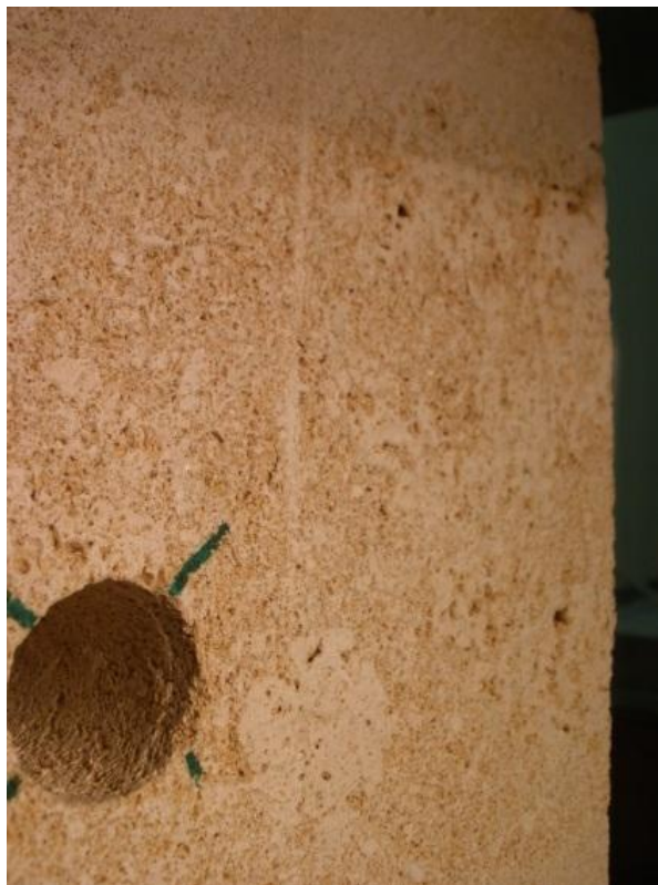
Fig.5.17: Cracks in specimen 12 for point 4 of the figure 5.11. Cracks on the side A of the specimen.
