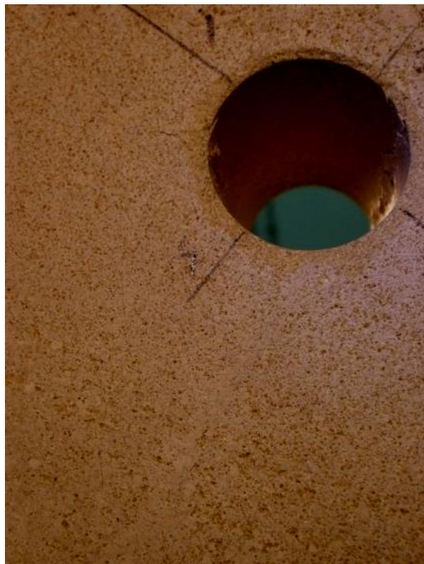
Fig. 5.42: Cracks in specimen 22 for point 2 of the figure 5.38. Cracks on the side B of the specimen.
