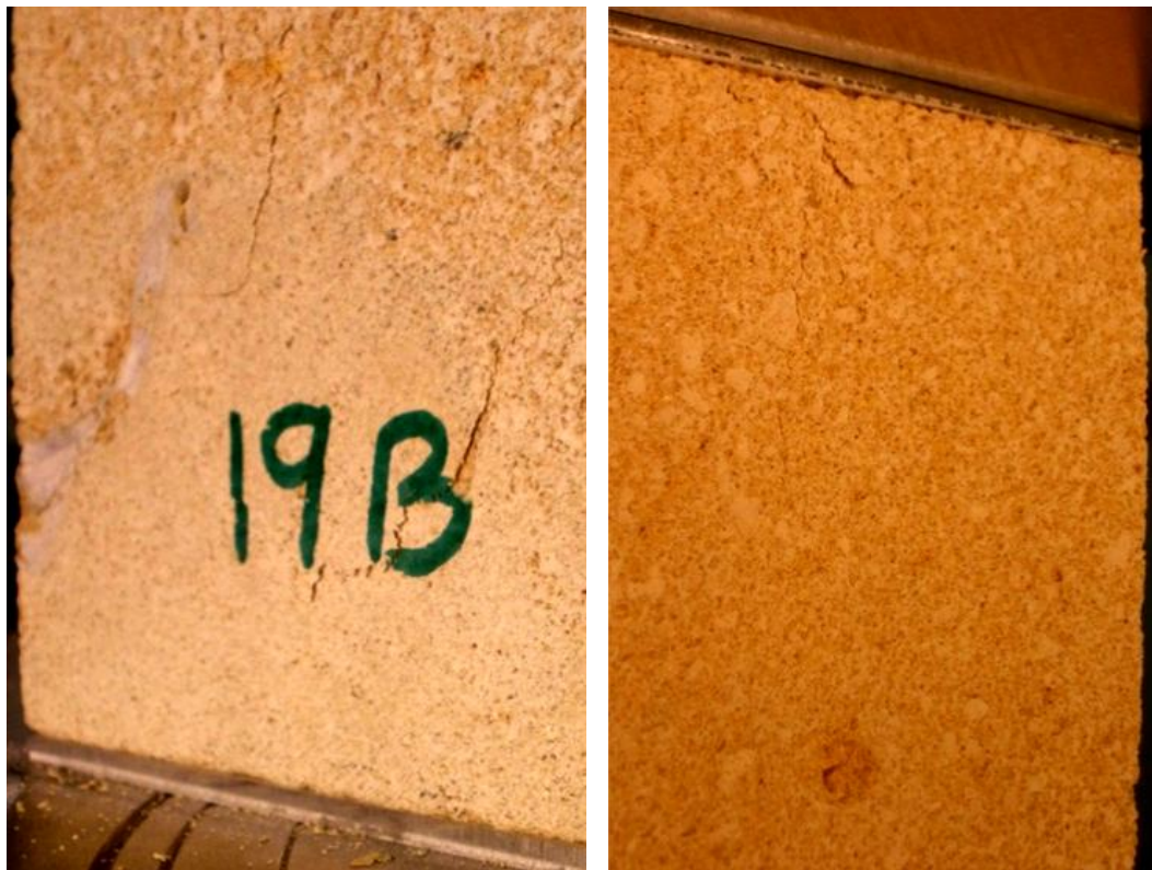
Fig. 5.32: Cracks in specimen 19 for point 8 of the figure 5.23. Cracks on the side B of the specimen.
