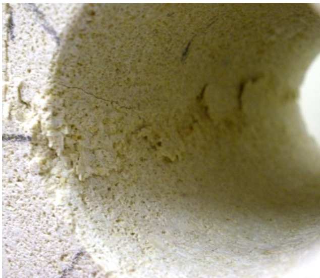
Fig. 9.26: Specimen 23 after testing. a) Side A. b) Side B. c) Drillhole of the specimen. The drillhole was photographed from side A.
