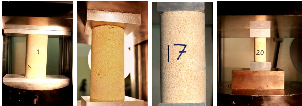
Fig. 5.55: Cylinder during test a) \Phi = 100 mm b) \Phi = 70 mm c) \Phi = 50 mm d) \Phi = 30 mm.
