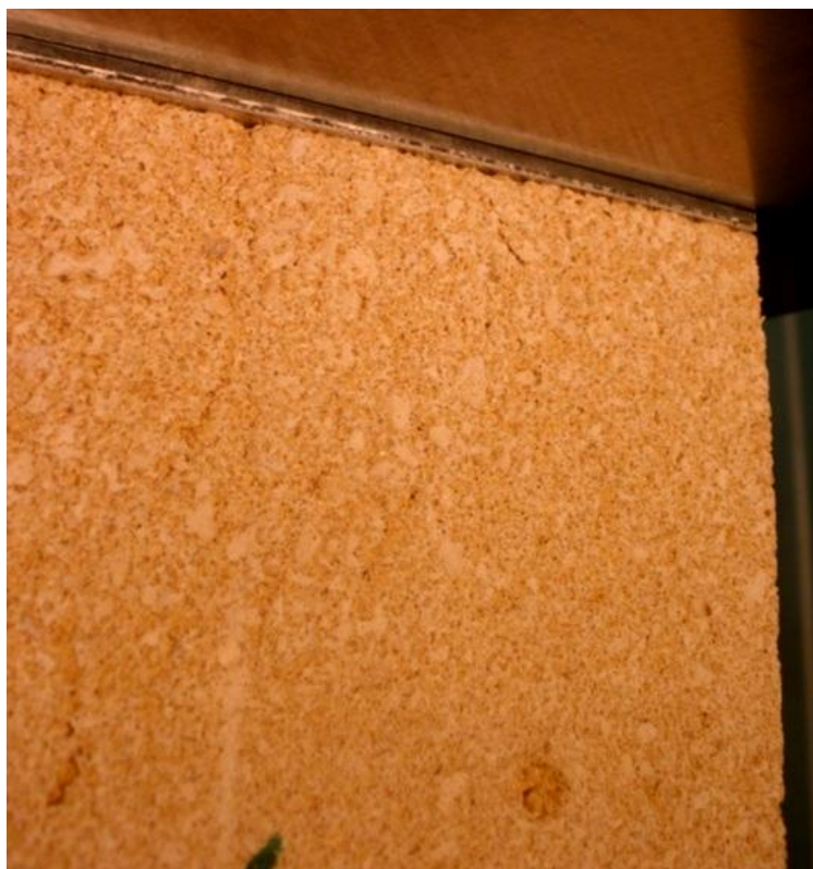
Fig. 5.27: Cracks in specimen 19 for point 4 of the figure 5.23. Cracks on the side B of the specimen.
