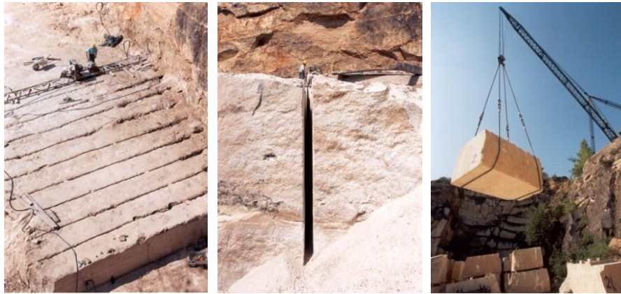
Fig. 5.2: Extracting technology in the quarry of St. Margarethen with a stonecutting machine. From: Gustav Hummel.
