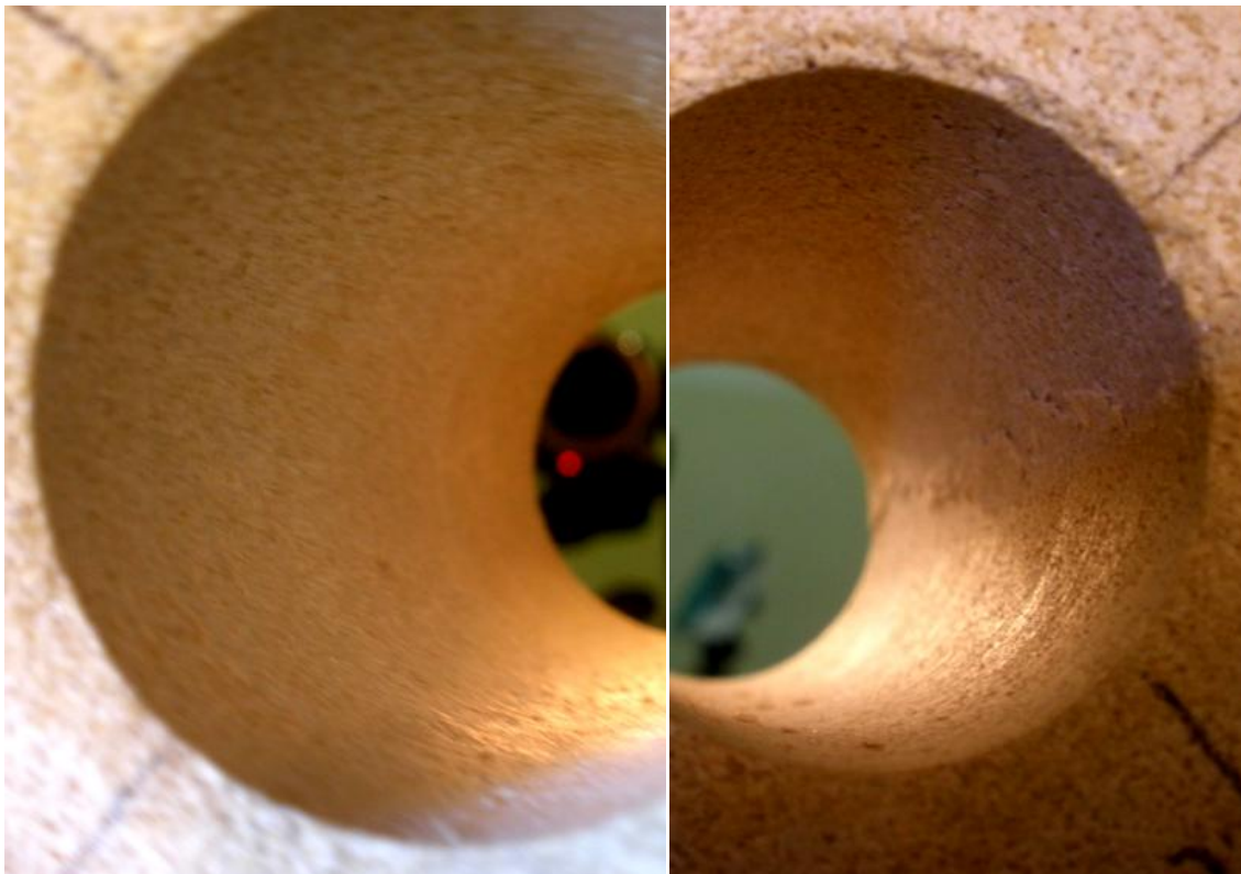
Fig. 5.39: Cracks in specimen 22 for point 1 of the figure 5.38. a) No rupture on the left wall of the drillhole. b) Rupture on the right wall of the drillhole. Picture was taken from side B of the specimen.
