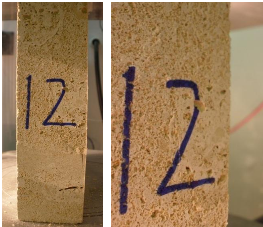
Fig.5.16: Cracks in specimen 12 for point 3 of the figure 5.11. Cracks on the right side of the specimen.
