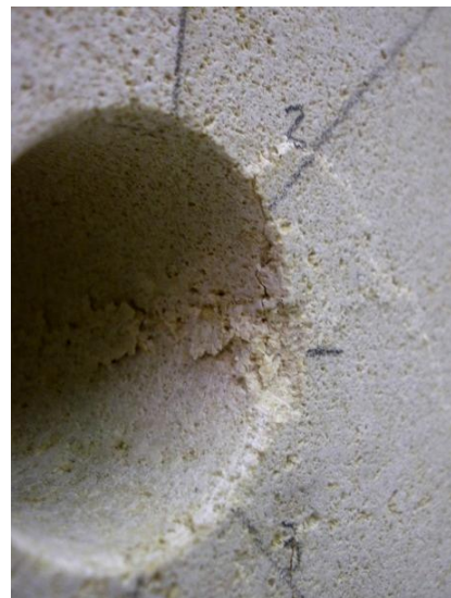
Fig. 9.26: Specimen 23 after testing. a) Side A. b) Side B. c) Drillhole of the specimen. The drillhole was photographed from side A.
