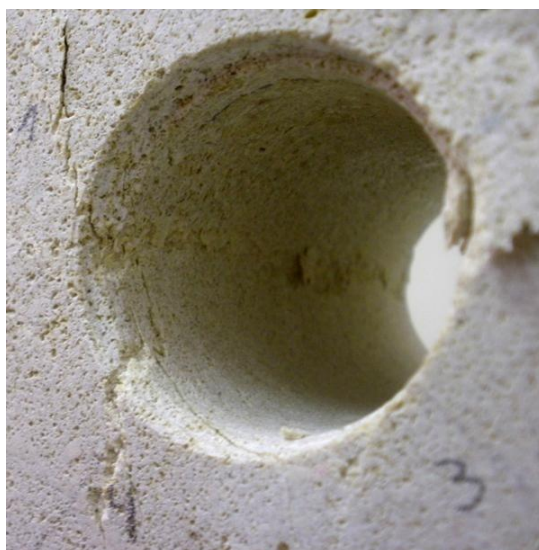
Fig. 5.48: Specimen 22 after testing. a) Side A. b) Side B. c) Drillhole of the specimen. The drillhole was photographed from side A.
