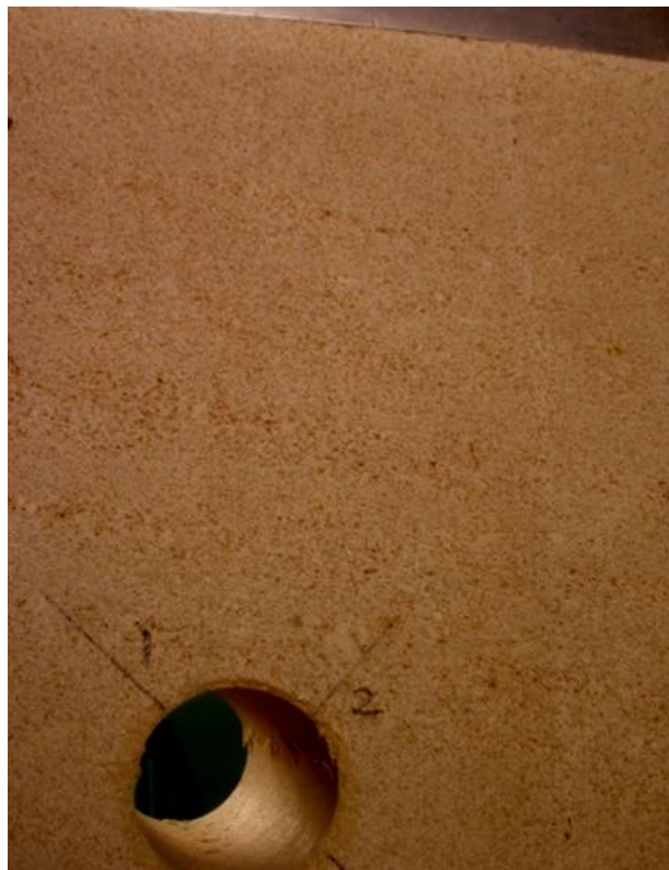
Fig. 5.43: Cracks in specimen 22 for point 3 of the figure 5.38. Cracks on the side B of the specimen.
