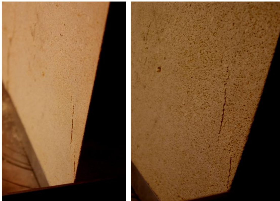
Fig. 5.46: Cracks in specimen 22 for point 5 of the figure 5.38. Cracks on the side A of the specimen.
