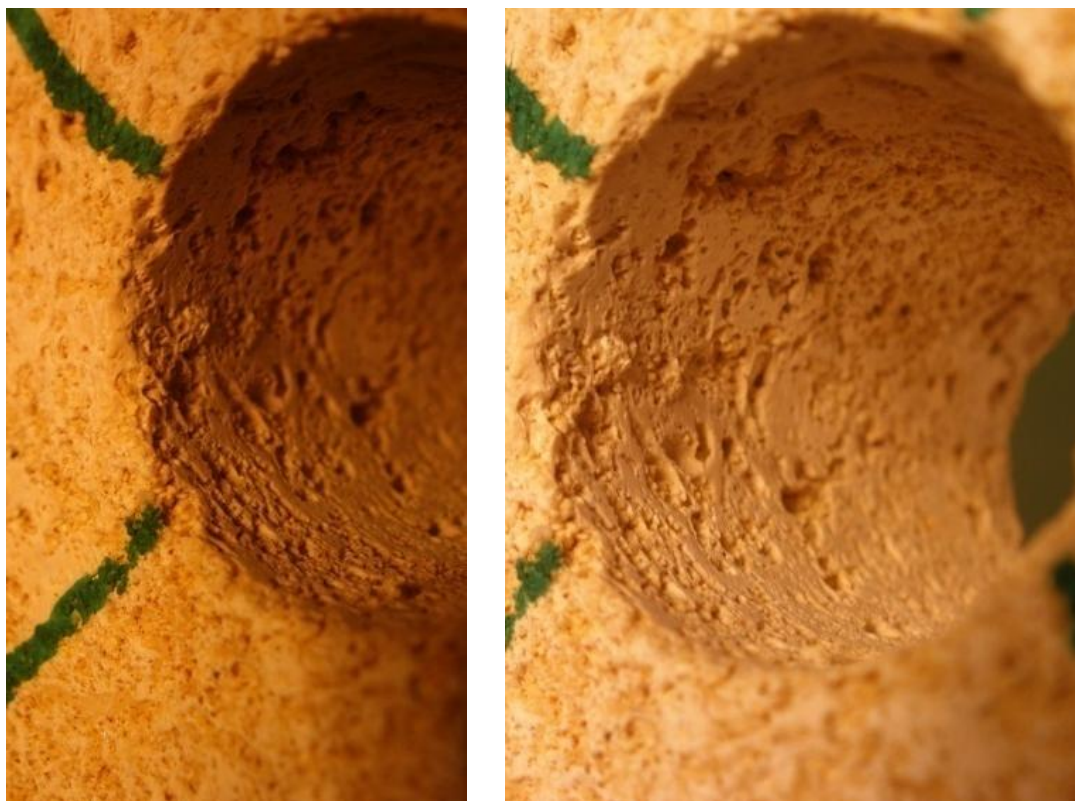
Fig. 5.15: Cracks in specimen 12 for point 3 of the figure 5.11. Rupture on the left wall of the drillhole.
