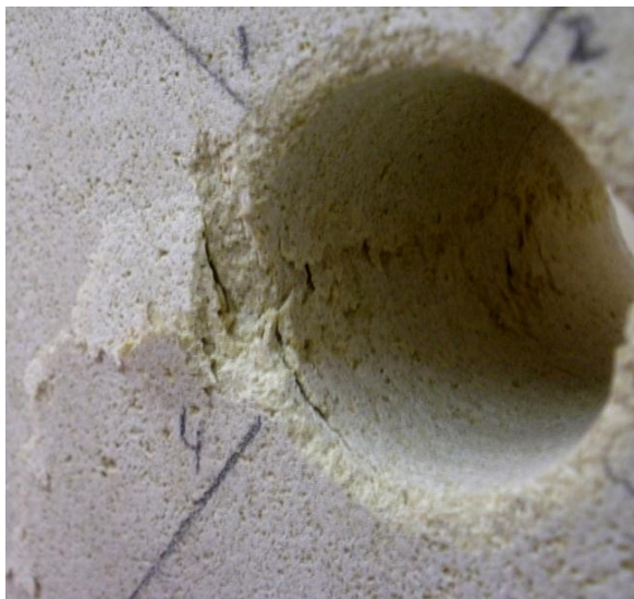
Fig. 9.23: Specimen 20 after testing. a) Side A. b) Side B. c) Drillhole of the specimen. The drillhole was photographed from side B.
