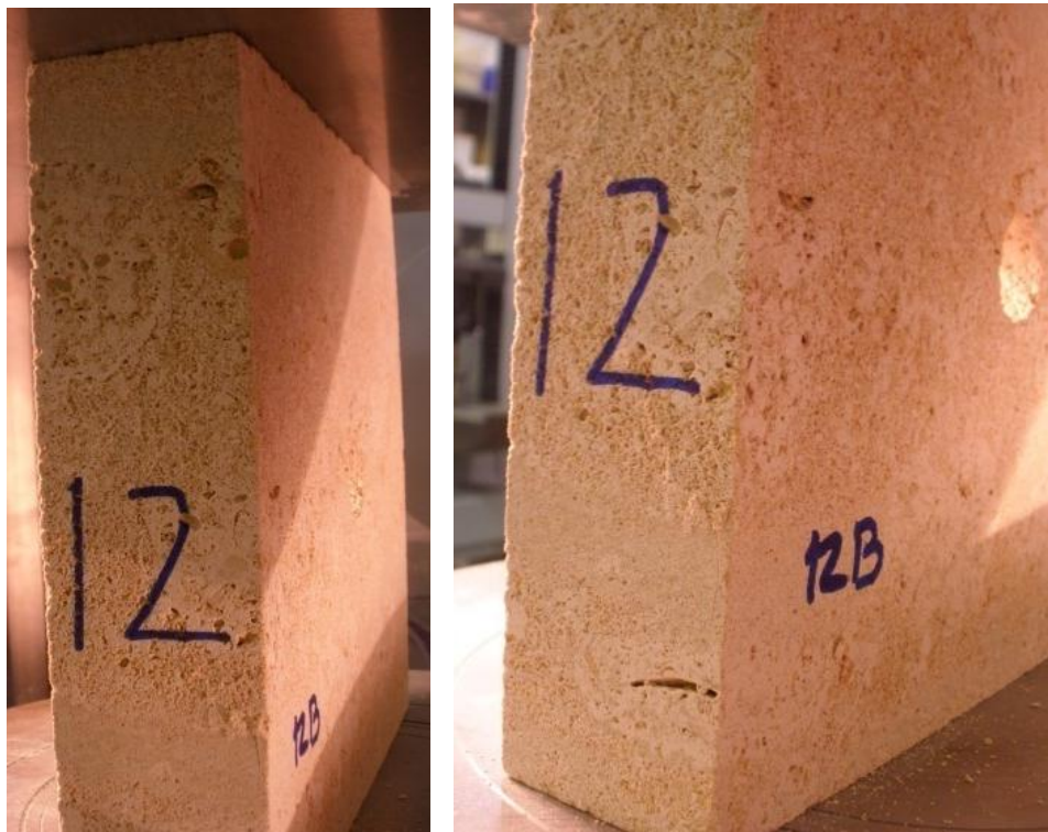
Fig. 5.12: Cracks in specimen 12 for point 1 of the figure 5.11. a) Cracks on right the side A of the specimen. b) Cracks on the side B of the specimen.
