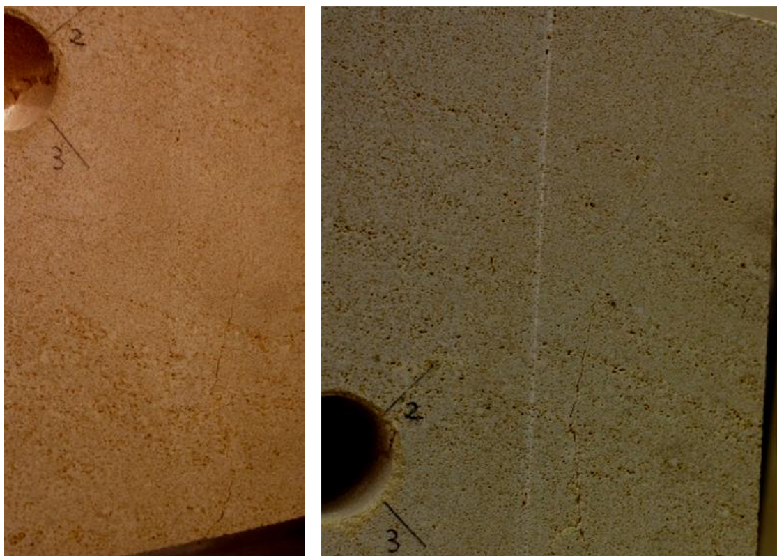
Fig. 5.45: Cracks in specimen 22 for point 4 of the figure 5.38. Cracks on the side A of the specimen.
