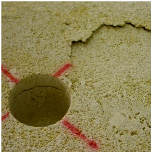
Fig. 9.14: Specimen 11 after testing. a) Side A. b) Side B. c) Drillhole of the specimen 11 after testing. (Left) The drillhole were photographed from side A. (Right) The drillhole were photographed from side B.
