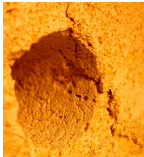
Fig.9.16: Specimen 13 after testing. a) Side A. b) Side B. c) Drillhole of the specimen. The drillhole was photographed from side B.
