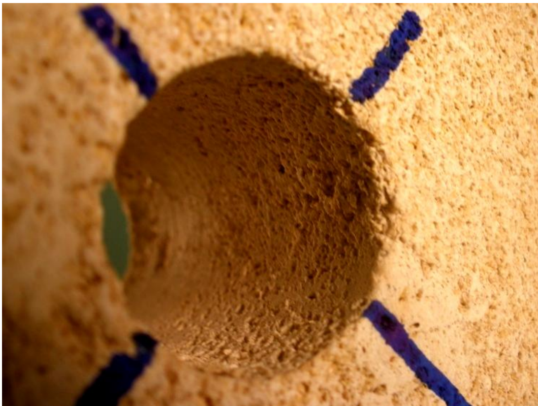
Fig. 5.29: Cracks in specimen 19 for point 6 of the figure 5.23. Rupture on the right wall of the drillhole. Picture was taken from side A of the specimen.
