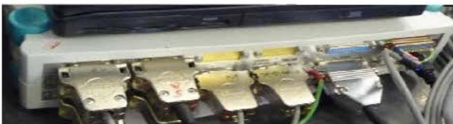
Abb. 4.17 Analog – Digital Signalwandler, Spider (HBM, 2009)
