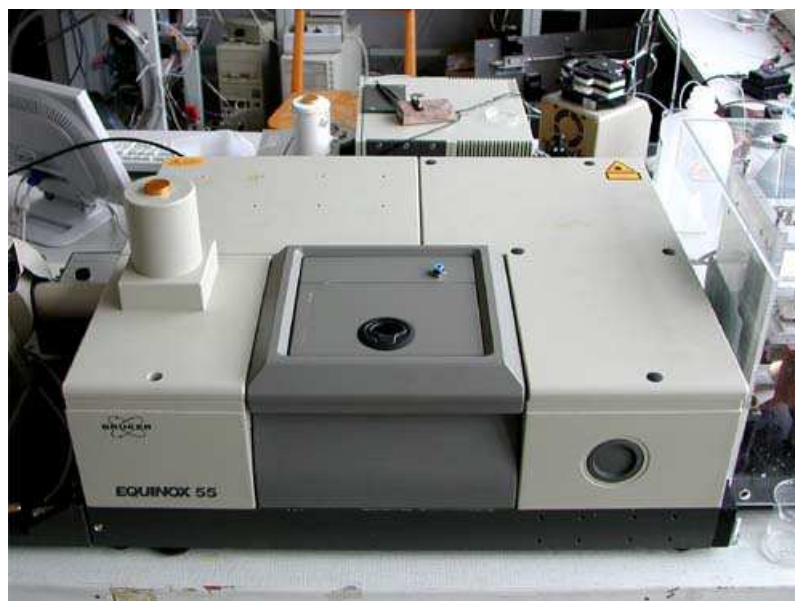
Figure 3.1: Example of a commercial FTIR spectrometer used in analytical chemistry (Bruker Equinox 55) [32]. Spectral range is 400-12000 \text{cm}^{-1} (0.83-25 \mu\text{m} ), spectral resolution is 0.20 \text{cm}^{-1} [33].
