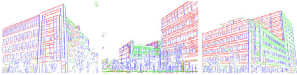
Figure 2.7.: Line-Based Structure from Motion: 2d line features are automatically detected by grouping edge pixels according to vanishing directions. Figure courtesy of [SKD06].
