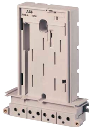
Figure 3.4: Interface for the ABB smart meter eHZ. With the help of this interface an non interruption exchange of the meter is possible. Source: ABB smart metering folder. With allowance of ABB.
