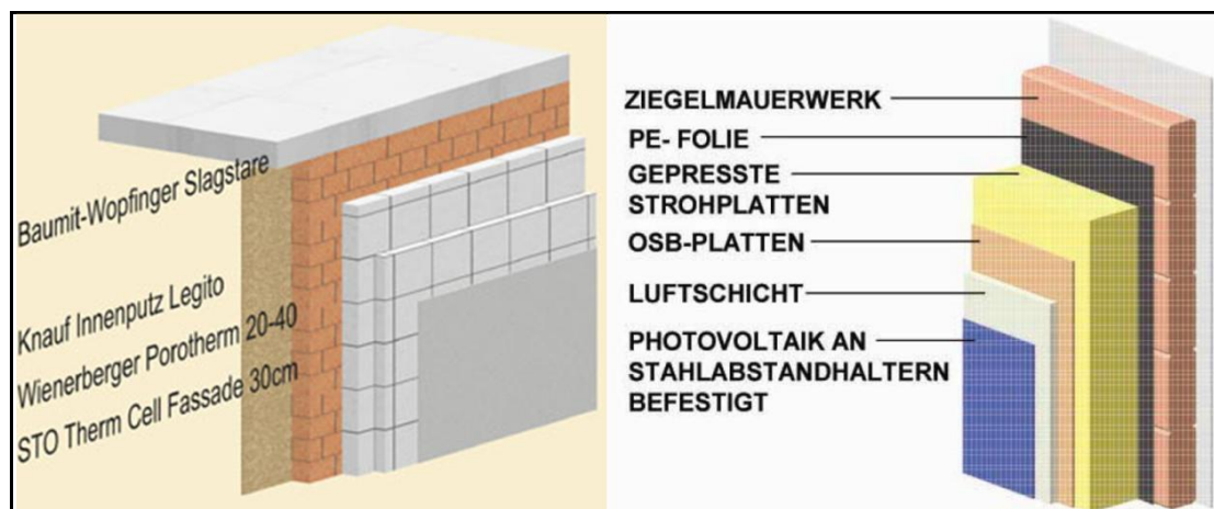
Figure III-17: Left image: Cement-free concrete ('Baumit-Wopfinger Slagstare') in combination with interior stucco ('Knauf Innenputz Legito'), brick masonry ('Wienerberger Porotherm'), and mineral foam board ('STO Therm cell Fassade').
