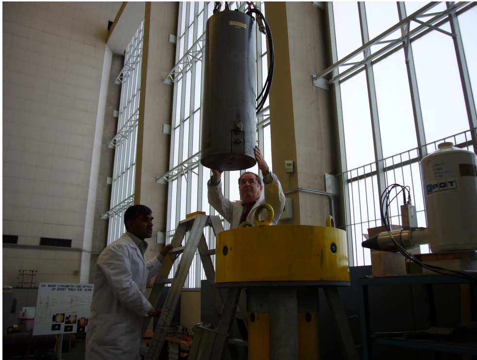
Figure 3.5: Fuel transfer to the fuel inspection unit at Atominsitute.
