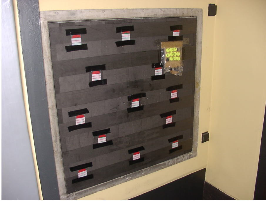
Figure 6.1: Graphite pile of stringers from the thermal column door side.
