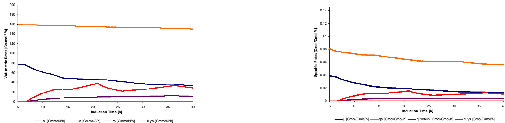
Figure 87: Fermentation at 20°C applying a linear feed ( k=0 ). Left: volumetric growth rate r_x (blue), volumetric substrate uptake rate ( r_s ), protein release rate r_p (purple) and volumetric cell lysis rate (red). Right: specific growth rate \mu (blue), specific substrate uptake rate q_s (orange), specific protein release rate q_{Protein} (purple) and specific cell lysis rate r_{Lys} (red). X-axis: induction time.
