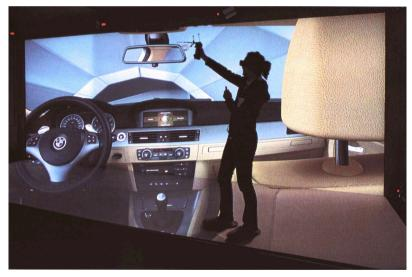
**Fig. 2.2** 2007: Powerwall (10x3m) in BMW research and innovation centre, Munich: high-end visualisation equipment (Kaltenbach, 2007, p. 1490).
