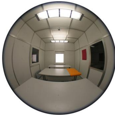
Figure 36 Operation of luminaire 1 for light output level 50% and daylight emulator for light output level 100%.
