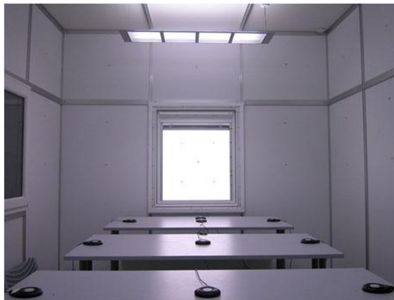
Figure 17 Internal view of the test room showing the sensors which measure horizontal illuminance for different dimming levels of the luminaires and the daylight emulator
