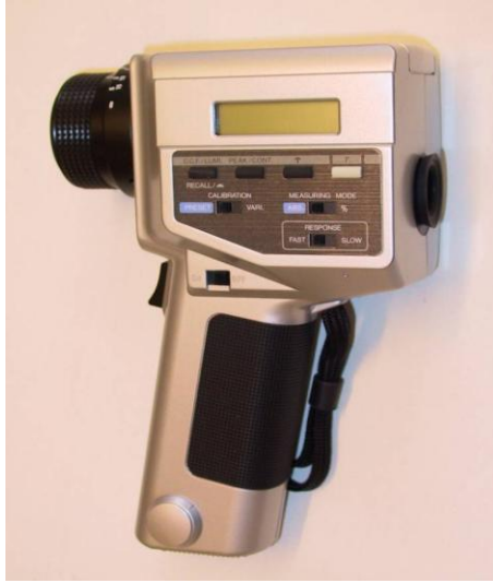
Figure 34 Instrumentation for the measurement of the luminance levels at various levels in the test room (desk, walls)
