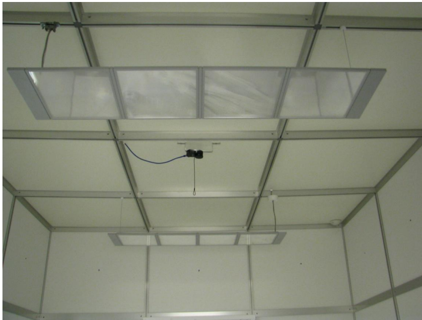
Figure 35 internal view of the testbed showing the camera used to measure the luminance levels on the desk.
