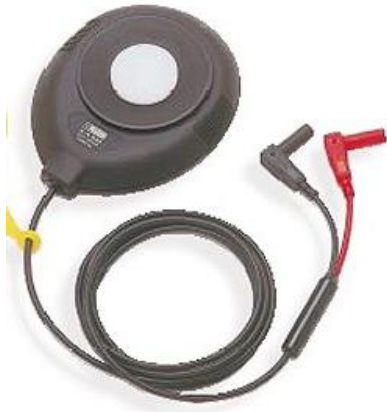
Figure 28 Instrumentation for the measurement of illuminance levels at 10 locations in the testroom.
