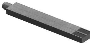
Figure 5.14: CAD-drawing of the used specimen holder<sup>31</sup>
