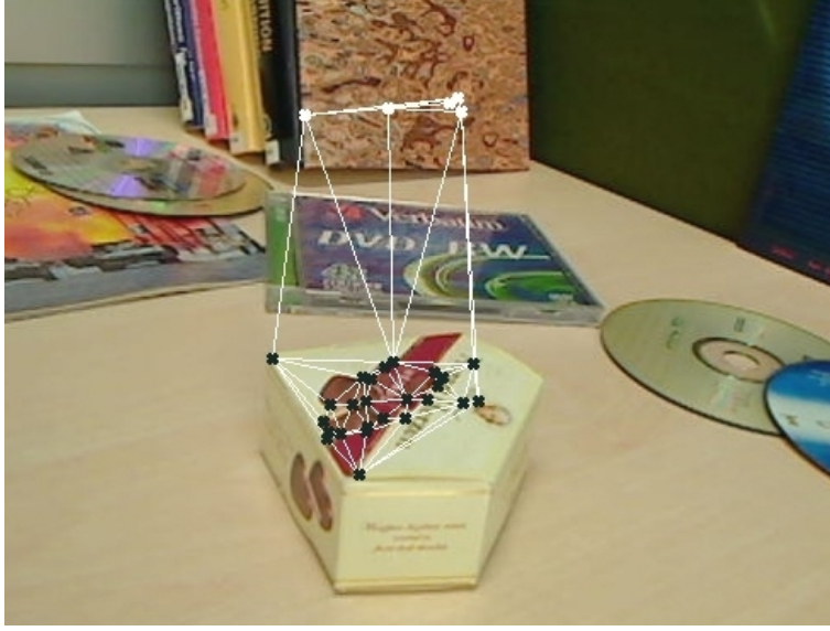
Figure 3.4: A plane (top surface of packaging) accidentally picks up interest points in the background. Therefore we split the interest point clusters (colored dots) using the mean and standard deviation of edges of a Delaunay graph (white edges).
