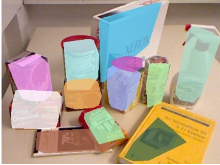
Figure 6.4: Typical scenario to test the object recognizer. The colored overlays are computed from the convex hull of the 3D points of the recognized object views, which are projected into the image.
