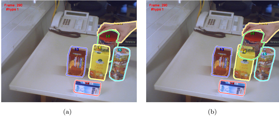
Figure 4.7: Two possible interpretations of an observed scene are shown. Figure 4.7(a) shows the best interpretation of the frame 290, which is the correct one. The confidence value of this hypothesis path is 0.9669, compared to the other interpretation in Figure 4.7(b), which is only 0.8913. The system explained the occlusion event correctly.
