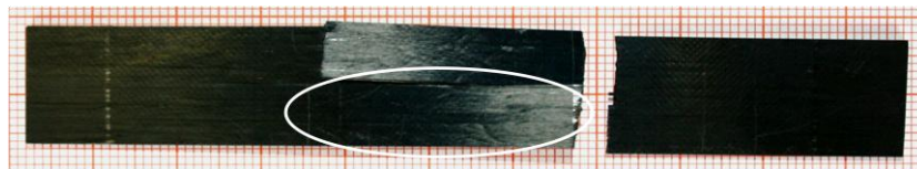
Fig. 4-4: Sample C3-4P-0-01 after four point bending showing the fragment investigated with SEM
