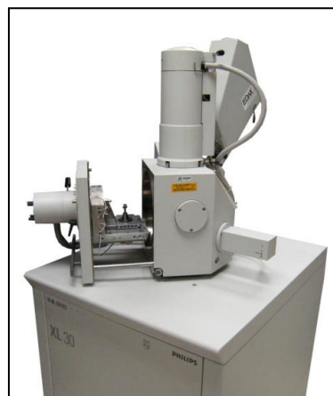
Fig. 3-7: Phillips XL 30 SE microscope [21]
