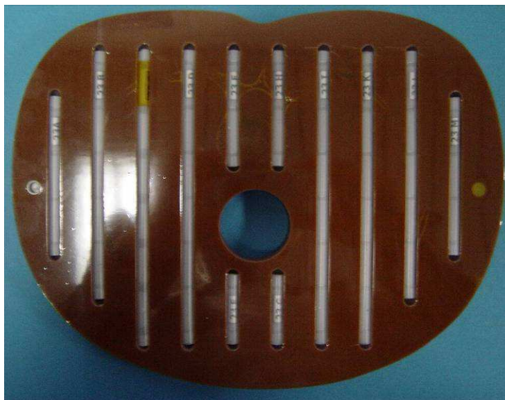
Fig. A.9. Distribution of detector tubes within the Matroshka phantom slice 23.
