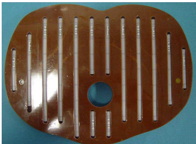
Fig. A.13. Distribution of detector tubes within the Matroshka phantom slice 31.
