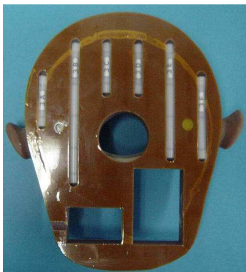
Fig. A.1. Distribution of detector tubes within the Matroshka phantom slice 3; cut-outs for integration of the eye organ box and a SSD.
