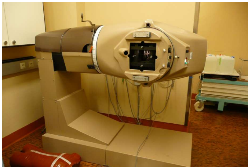
Fig. 3.1.1 ^{60}\text{Co} source with pneumatic shutter (Philips Theratron) [source: ATI].
