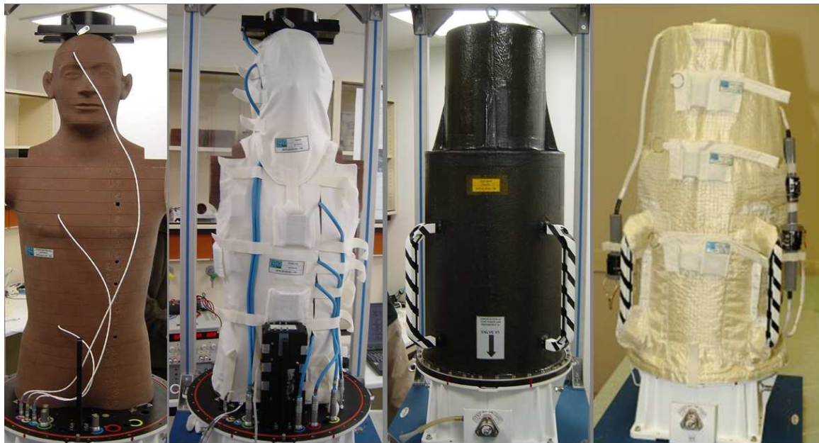
Fig. 1.4.4 from left to right: the phantom torso divided into 33 slices, the hood, the containment and the MLI.
