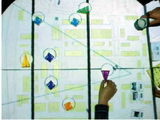
Figure 4.2.: A-Tokens of the ColorTable that the sensing technology captures: 2D positions, sizes, shapes and colors
