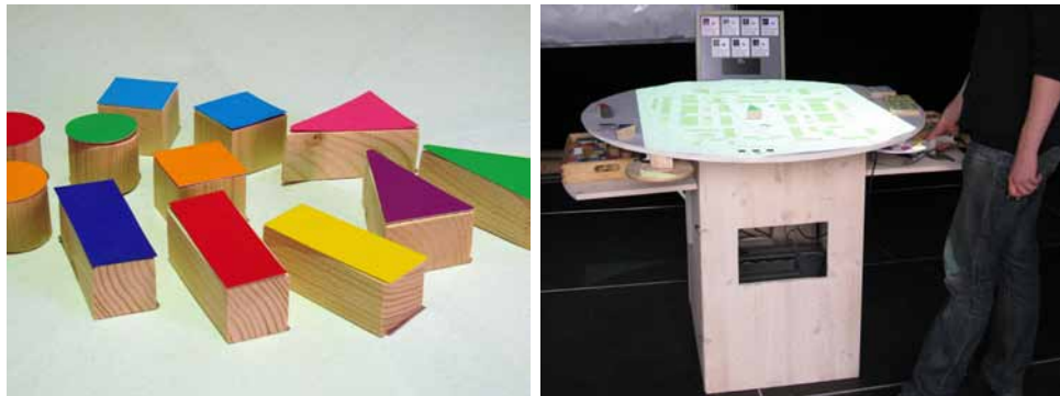
Figure 8.10.: Re-designed color tokens (left); physical ColorTable including rotating disk, tangible selector and retractable side frames (right).
