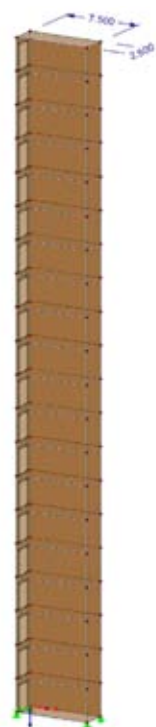
figure 5.2: Calibration of the 2. natural frequency for timber core in RSTAB and RFEM
