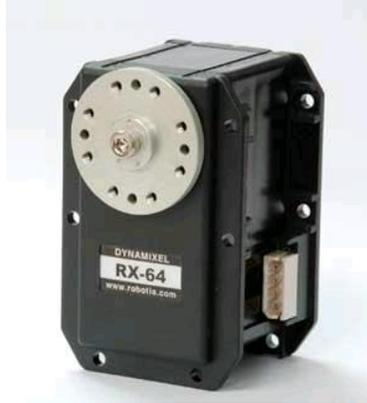
Figure 5-1: RX-64 servo motor used in Archie
