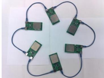
Figure 5-21: Daisy chain network for spreading the communication bus in the robot
