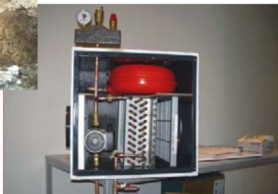
Air-to-air subsoil Winter heat exchanger vs. Liquid-to-air subsoil heat exchanger for Summer cooling
