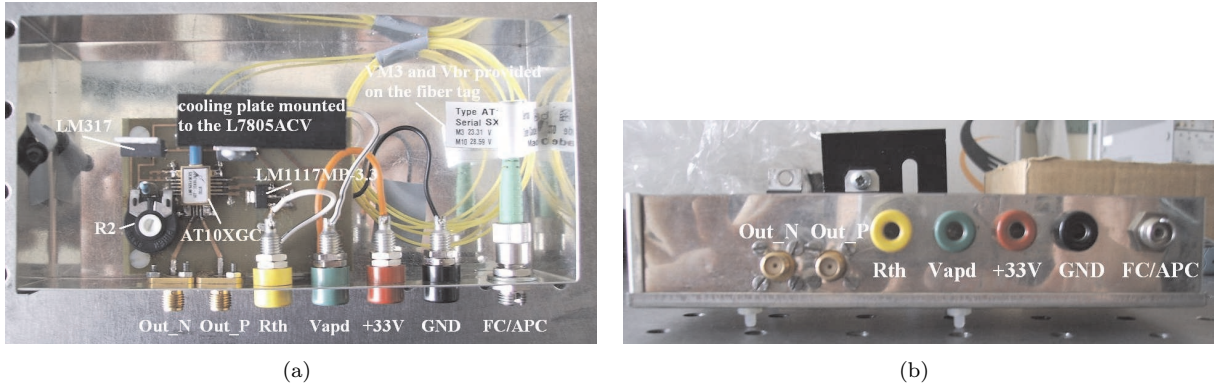
Figure 2.15: The fully assembled APD AT10XGC in its housing a) top view b) front view.
