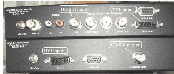
Figure 3.18: Backside of the DVI HD-SDI signal converters.
