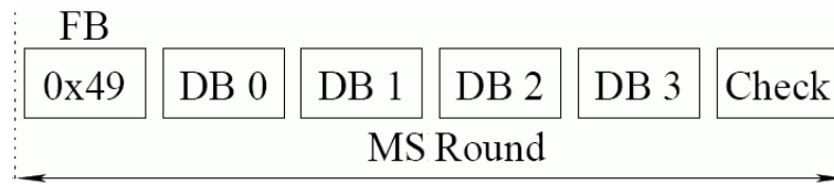
Figure 2.13: Structure of a TTP/A Master – Slave Round[EHK + 02]
