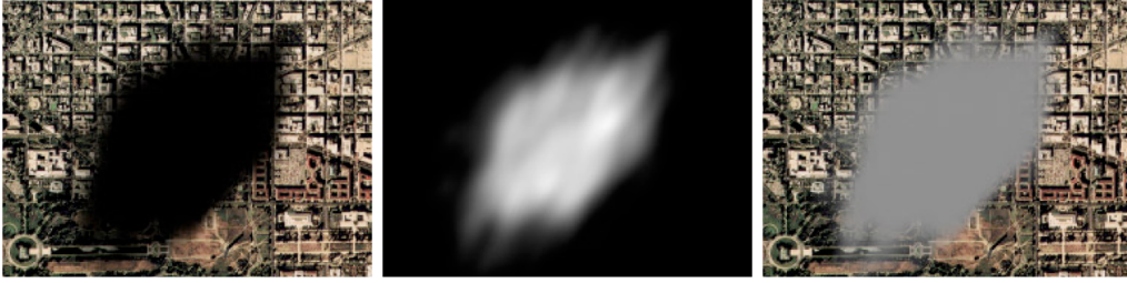
Figure 2.4: Three different optical models. From left to right: absorption only, emission only, emission and absorption. [51]
