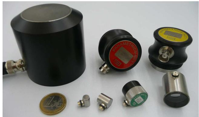
Figure 3.10: Ultrasonic transducers
