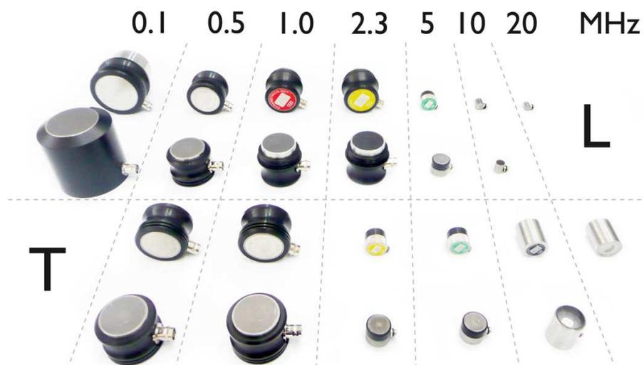
Figure 1.1: Examples for used ultrasonic longitudinal ( $L$ ) and transversal ( $T$ ) transducers.
