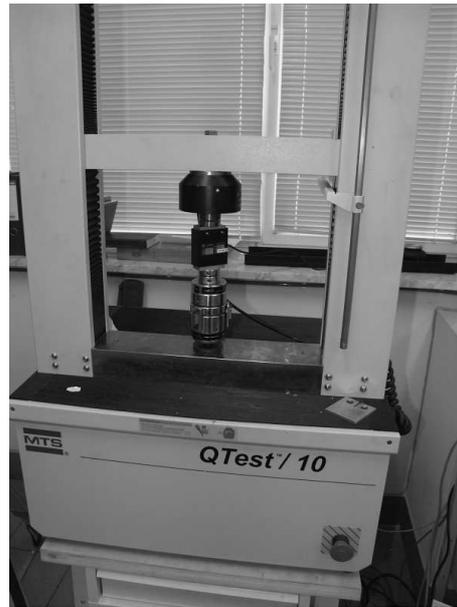
Figure 5.7: Electromechanical testing stand for compression tests on CEL2-based biomaterial samples
