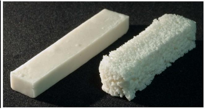
Figure 3.6: CEL2 glassceramic samples (left dense, right porous)
