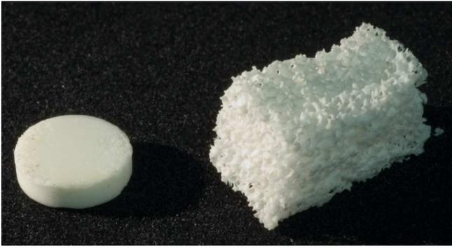
Figure 3.5: Bioglass<sup>®</sup>-ceramic samples (left dense, right porous)
