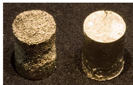
Figure 3.2: Titanium samples (left porous, right dense)
