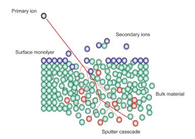
**Figure 2.1:** Fundamental principles of the secondary ion formation (illustration from company-internal documents of Ion TOF, Germany)
