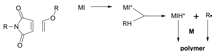
Scheme 11. Structures of maleimide/vinyl ester system and schematical initiation process
