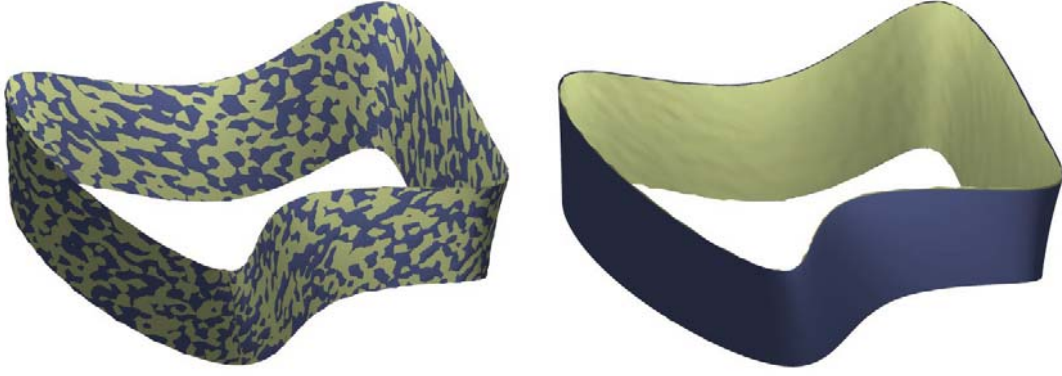
Figure 6.2: (Left) Least-squares approximation (blue) of a target shape (yellow). (Right) undercut free and one-sided approximation of the same setup. The target shape has been triangulated for better visualization.
