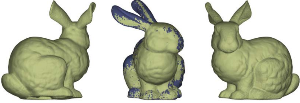
Figure 4.2: A reconstruction of the Stanford bunny model from more than 300 simulated noisy scans. The original model is included as ground truth (blue) in the center figure. The point clouds have been triangulated for better visualization.
