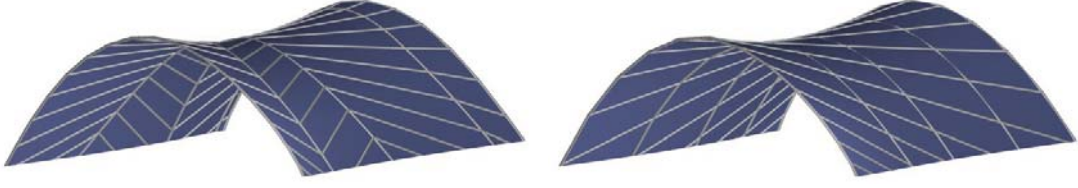
Figure 6.10: Smoothing of polygonal rulings lines (right) yields a visually more pleasing ruled surface strip reconstruction than an unconstrained approximation (left).
