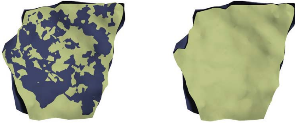
Figure 3.7: Unconstrained registration (left) yields a final alignment with mutual penetration of target and moving point cloud. The inclusion of linear constraints — eventually simplifying the smooth variant of the point to tangent plane l_1 -registration — achieves a penetration free alignment (right).
