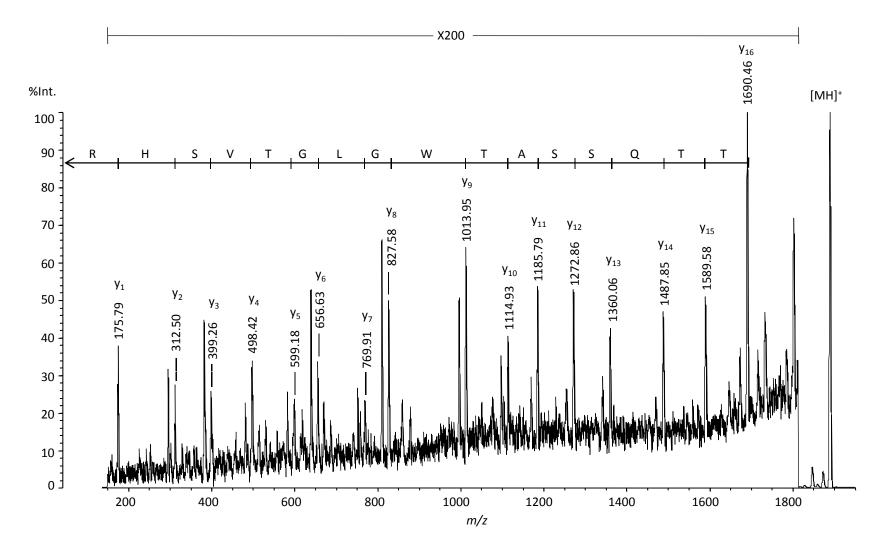
*Figure 4*. MALDI PSD spectrum obtained from the precursor ion at m/z 1888.9 after *on-target* tryptic digestion of *Fusarium* macroconidia spores.
