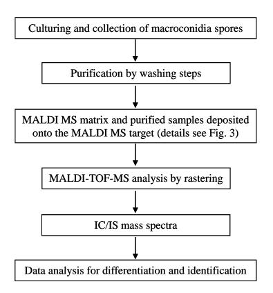
*Figure 2*. Strategy of intace cell/spore mass spectrometry (IC/ISMS) of *Fusarium* macroconidia.
