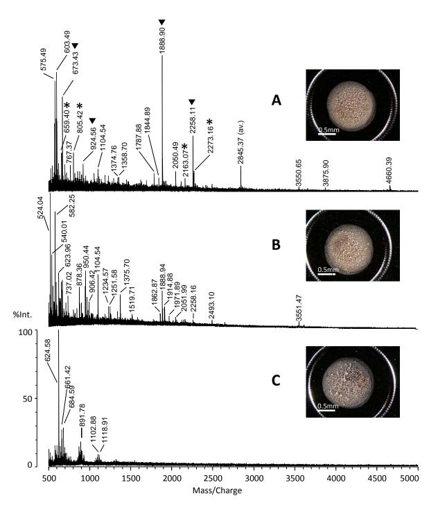
**Fig. 3.** MALDI TOF mass peptide mass spectra of *Giberella* strain 2985 with *on*-*target* digestion using (A) non-immobilized trypsin and (B) immobilized trypsin as well as (C) without enzyme (the applied MALDI MS sample preparation in this case is not useful for ICMS). Trypsin autodigestion peaks were marked with \* and the selected peaks for PSD fragment ion analysis were marked with  $\blacktriangleright$ .
