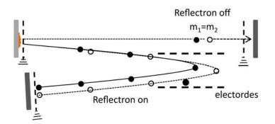
Figure 2.2 Principle of an RTOF mass analyser
