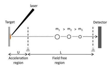
Figure 2.1 Principle of an LTOF mass analyser
