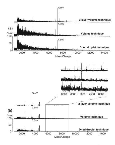
Fig. 6 Comparison of MALDI mass spectra of intact Fusarium conidia pores using different matrix solution/conidia spore solution ratios applied with twolaver volume technique (a, left column) F. poae strain 2786 (light-colored) and (b, right column) F. graminearum strain 2765 (deep-colored). Matrix solution, 10 mg ferulic acid dissolved in 1 mL ACN/0.1% TFA (7/3, v/v); washing solvent system: ACN/0.5% FA (7/3, v/v); matrix solution/ conidia spore solution mixing time, 3 min
