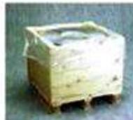
05 Coils with centre support separated by cardboard
