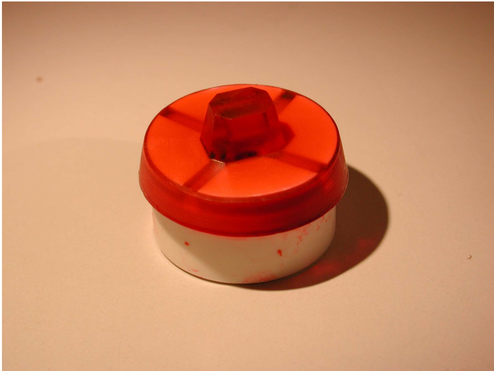
Figure 1.1: A prepared and hardened block ready for the following sectioning on the microtome.
