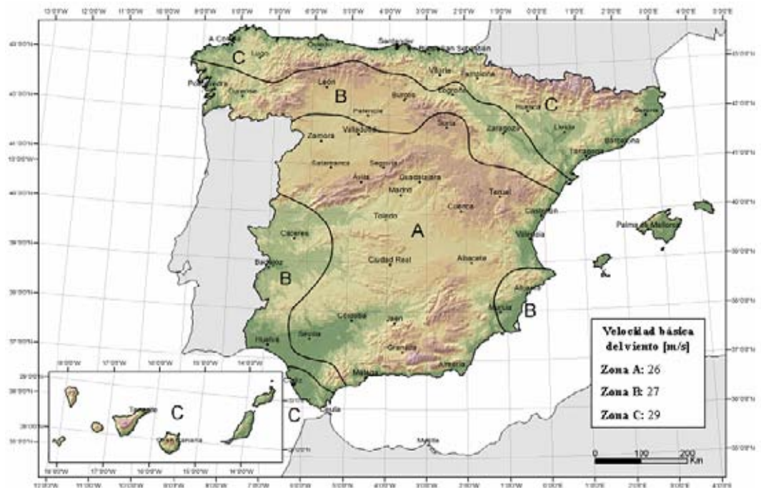
Figure B.4 Basic Value of the wind speed in Spain (CTE-DB-SE-AE march 2006)
