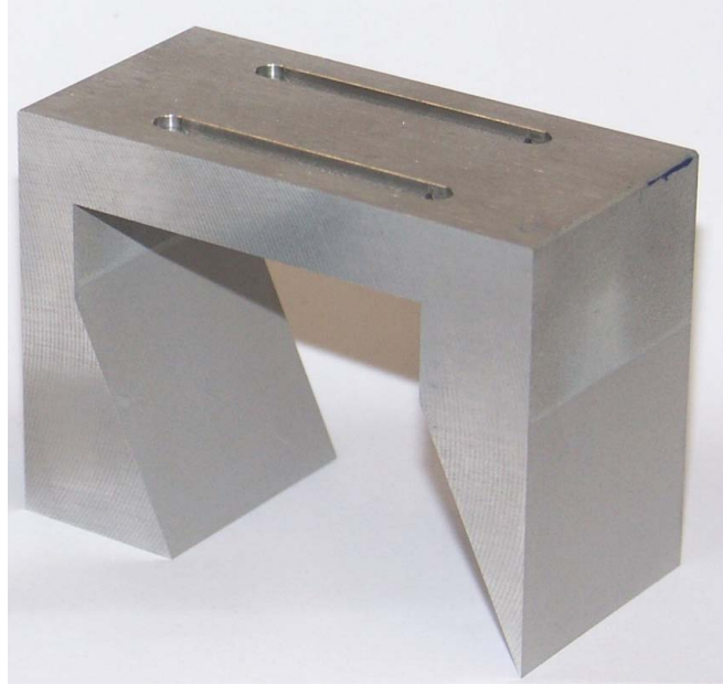
Figure 6.8: Connected set of two 25° aluminium prisms, that are cut from one aluminium block.
