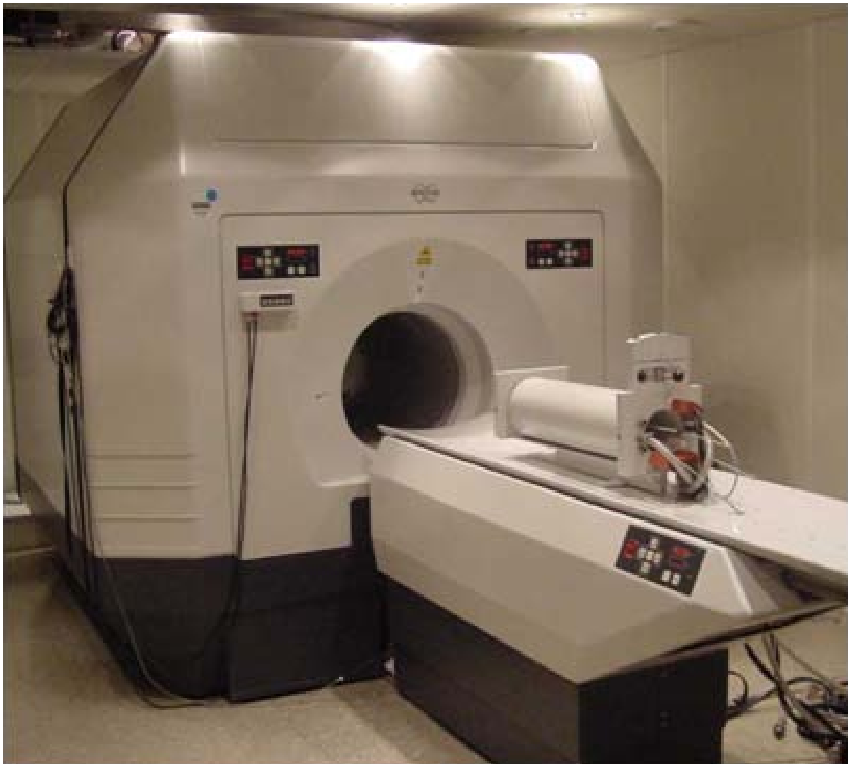
Figure 3.02: Bruker Medspec 30/80 with actively shielded micro-imaging gradient system BGA-12
