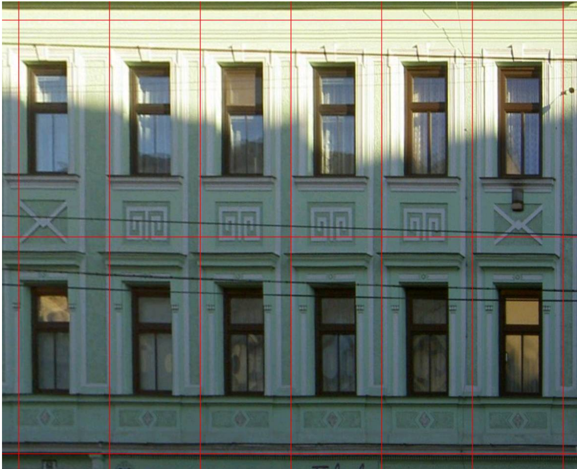
Figure 2.1.: Window tile segmentation on partially shadowed facade (detail). The computed segmentation is illustrated by red lines superimposed on the original image. The segmentation is not obscured by shadowing or other potentially disturbing image artifacts (see chapter 3).
