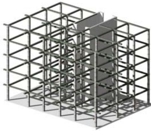
Figure 3-8: Skeleton reinforcement structure approved
