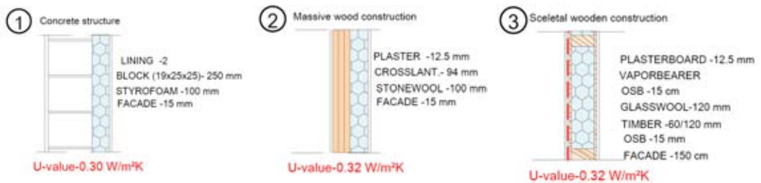
Figure 7-4: Composition of outer walls for the four Buildings
