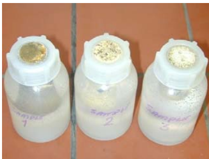
Figure 5-9 Left: Permeability measurement. The stones are hermetically sealed in vessels completely filled with water. Then the evaporation through the outer surface was measured over a time
