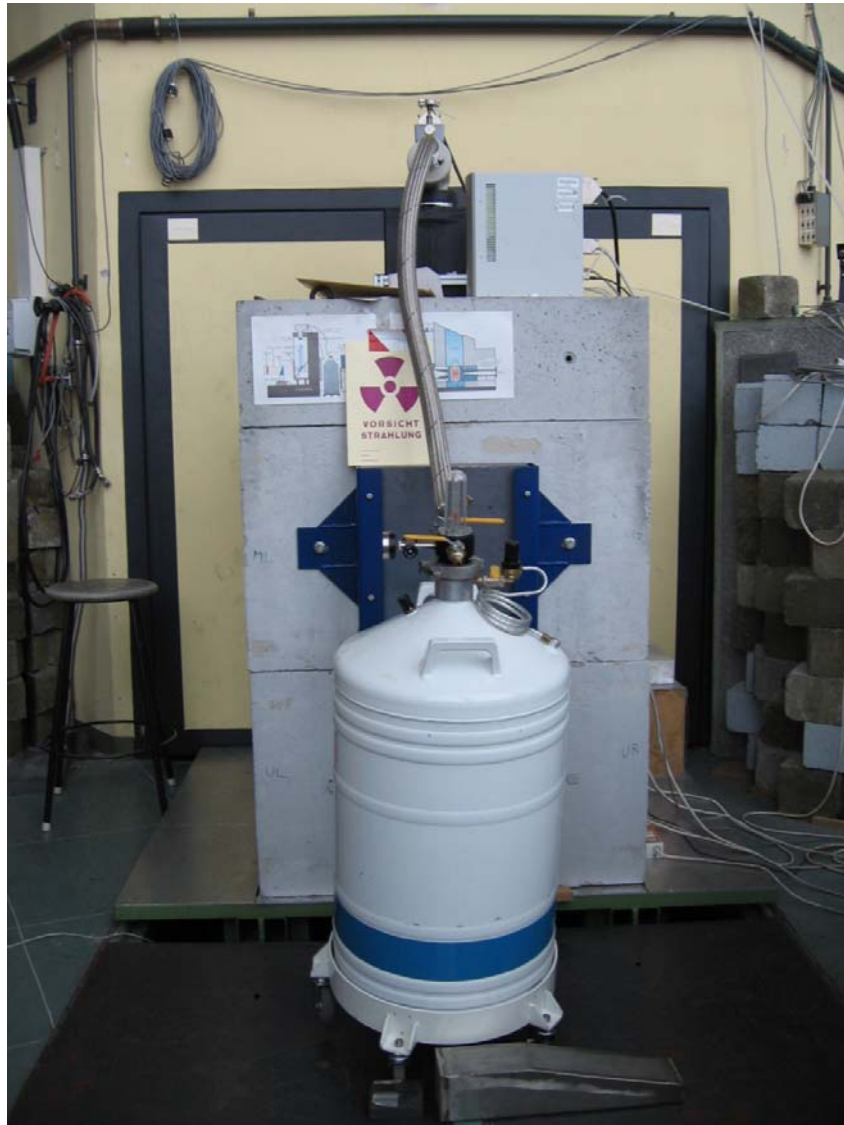
Figure 4-10: Nitrogen filling for cooling the CCD camera.
