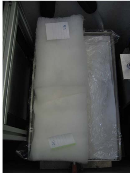
Photo at the end of the experiment. The CLY fibers seem to have collapsed.
