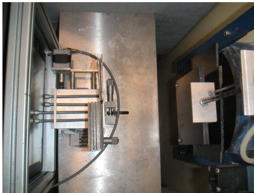
Figure 10-5: Neutron radiography measurements of different thicknesses of the boron steel plates were made using the scintillator detector. The distance between the detector and the sample was also varied.
