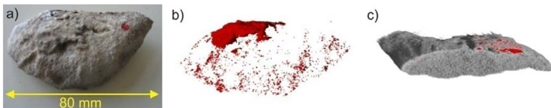
Figure 13-2: a) Photograph of the sample. b) NT of the sample. The stone has been made transparent to reveal the highly attenuating regions.
