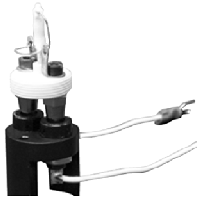
Figure 4.4: The LSB151 30W infrared element from LOT Oriel.
