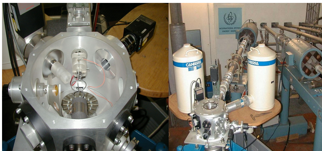
Figure 5. (a) The Scattering Chamber (b) The IAEA PIXE beamline
