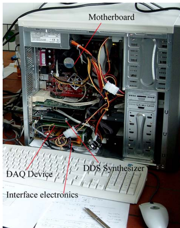
Figure 7: Picture of the PC version of the QxSens system. The important parts for the QxSens system are marked.
