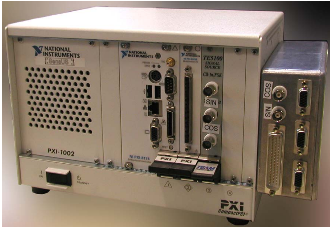
Figure 8: Picture of the PXI version of the QxSens system. The interface electronics are mounted on the right side of the chassis.
