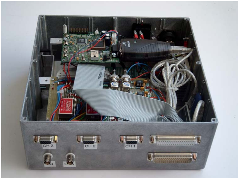
Figure 9: Picture of the open housing of the external USB version of the QxSens system.
