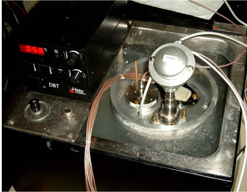
Figure 57: Three sensors mounted in a specially developed metal housing, that is put in a water bath. This measurement system is used for calibration of QV sensors.
