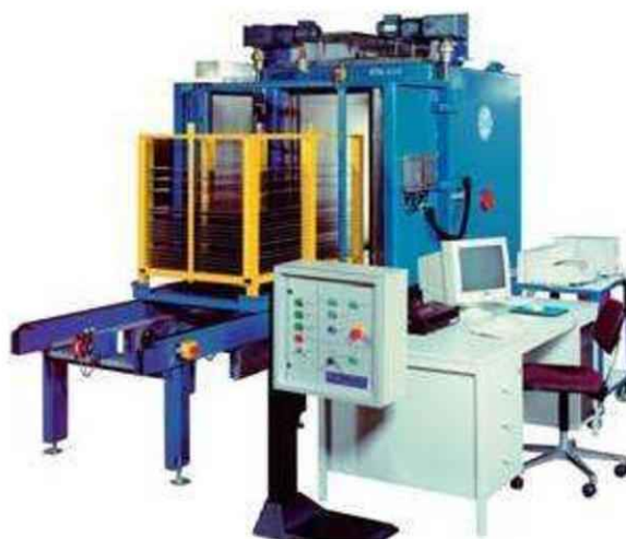
Figure 3.2: Photograph of the clearance measuring system RADOS RTM644Inc, PSI, Villigen (CH)
