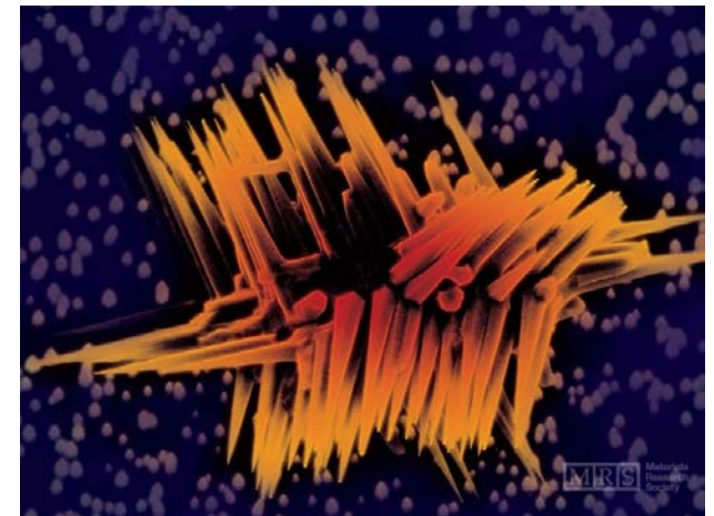
Fig.5.9. Highly tapered germanium nanowire grown from a surface imperfection, utilizing the vapor-liquid-solid mechanism on an Si (111) substrate. Imaged via field emission SEM at a magnification of 15k, accelerating voltage of 5 kV, and imaged in plan view, normal to the (111) substrate surface.Credit: Teresa Clement, Arizona State University
