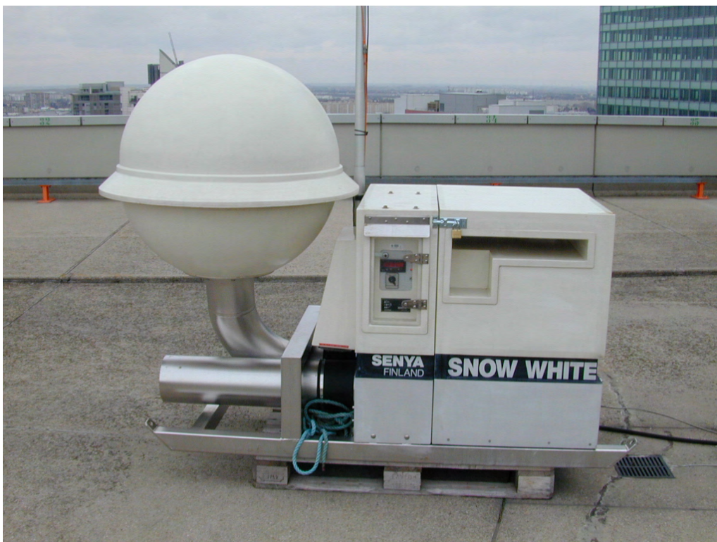
Figure 34 Snow White JL-900 air sampler installed at the Vienna International Centre
