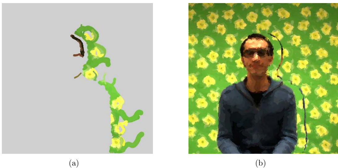
FIGURE 7.4 The strokes are allowed to emanate from the unmasked pixels in the occlusion map to masked pixels. The result of this constrained progressive painting (with 3 layers) is shown in Figure (a). Inaccuracies in the disparity map, in particular foreground object boundary expansion, produce a right stereo component after image warping that has noticeable defects, as shown in Figure (b).
