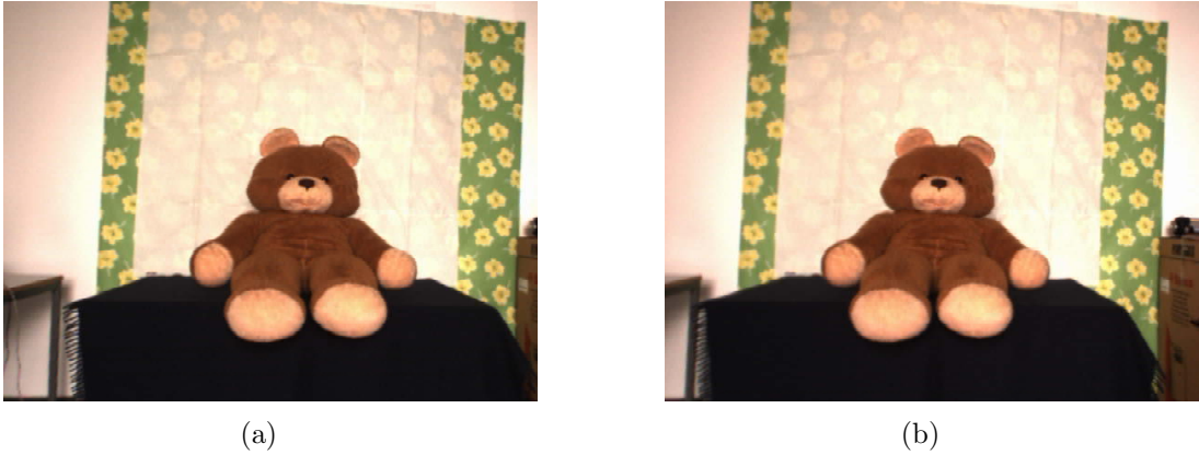
FIGURE 4.2 The “Brown Teddy” dataset shown here is an example stereoscopic image pair captured by our calibrated camera system. Figures (a) and (b) show the left and the right stereoscopic components after rectification, respectively.
