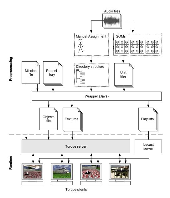
Figure 5.1: System architecture.
