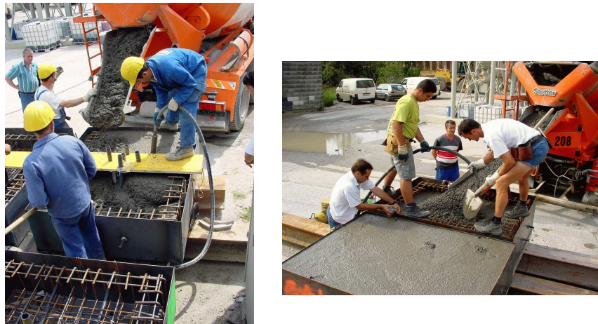
Figure 2.32: Casting of large-scale specimens for fire experiments under on-site conditions [67]
