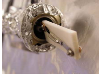
Figure 3.14: Picture of the home-built potassium dispensers
