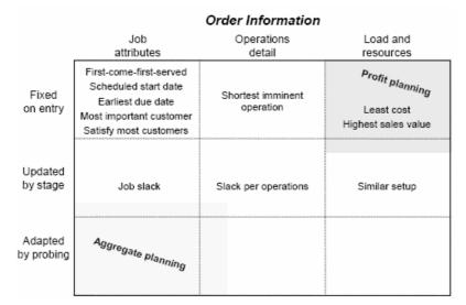
figure 19: classification of the dispatch priority rules (slack = time left from current time to due date)
