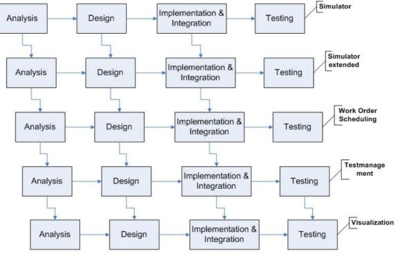
figure 21: incremental software process (SAW project)
