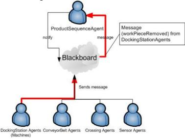
figure 16: Interaction in Blackboard Pattern - Docking Stations and PA
