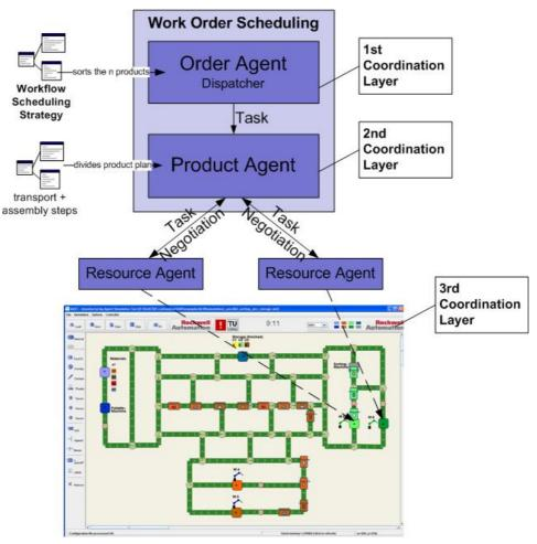
figure 29: Coordination layer model of the project
