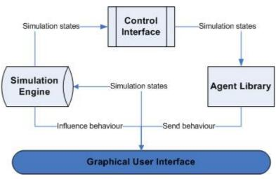
figure 22: Simulator Architecture
