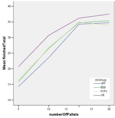
figure 26: number of finished product in contrast to number of pallets
