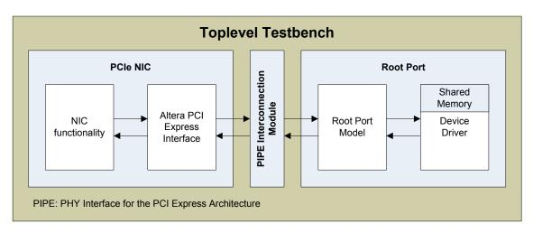
Figure 6.1: Architecture of the Altera simulation environment
