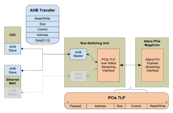
Figure 3.1: Register read and write operation
