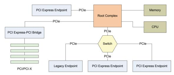
Figure 2.8: Example topology of a PCI Express architecture
