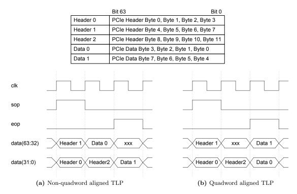
Figure 2.13: Mapping of 32-bit addressed PCI Express TLP to Avalon ST bus
