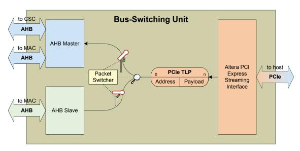
Figure 3.5: Operation principle of a separate switching module
