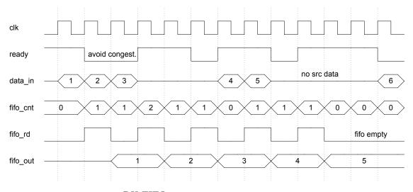
Figure 5.6: RX-FIFO timing with intelligent ready signal control
