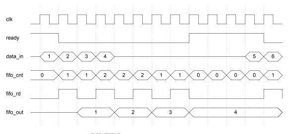
Figure 5.5: RX-FIFO timing with simple ready signal control
