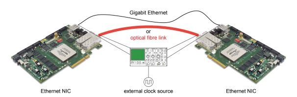
Figure 1.4: Example setup for delay measurements
