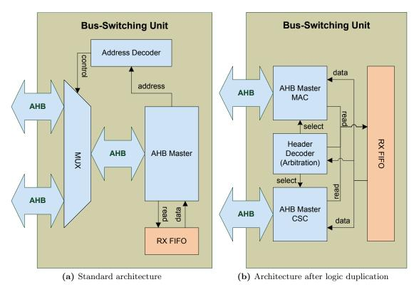
Figure 5.7: Address decoding with one and two AHB masters
