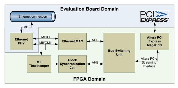
Figure 4.2: Module interfaces and hardware domains of the NIC
