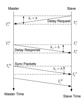
Figure 2.14: Synchronization messages and round-trip delay measurement
