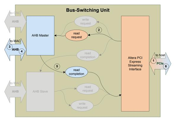
Figure 3.2: Information flow in the bus-switching unit for register operation
