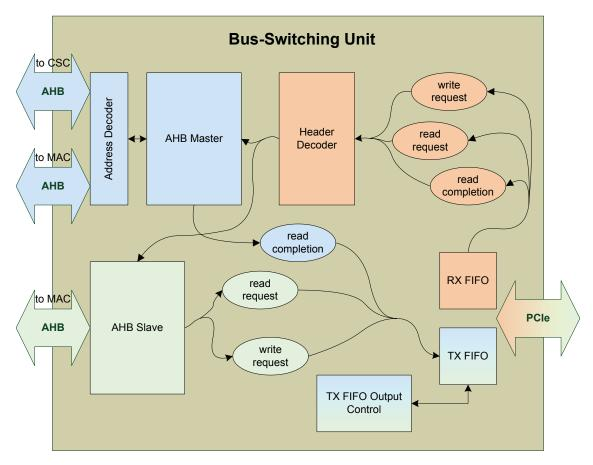
Figure 5.4: Architecture of the bus-switching unit
