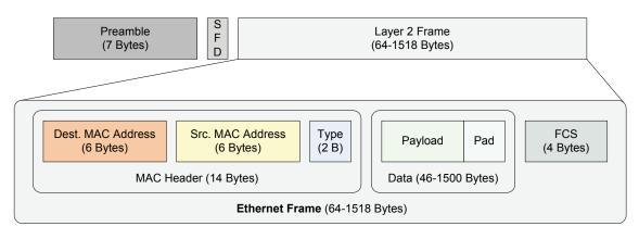
Figure 2.2: Structure of a standard Ethernet packet neglecting extensions
