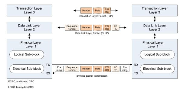
Figure 2.9: Three layered architecture of PCI Express
