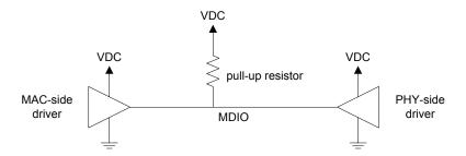
Figure 5.2: Pull-up resistor and drivers of the MDIO bus line
