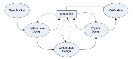
Figure 5.1: Typical design flow
