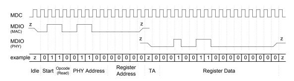
Figure 2.5: Timing and structure of a MDIO frame
