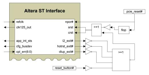
Figure 5.3: Reset circuitry for the PCI Express Endpoint
