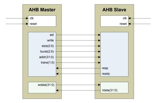
Figure 2.6: AHB lite master and slave interface signals
