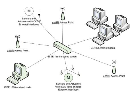
Figure 1.3: Example network for clock synchronization
