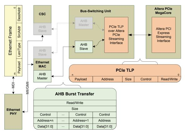
Figure 3.3: Ethernet over AHB-burst-transmission
