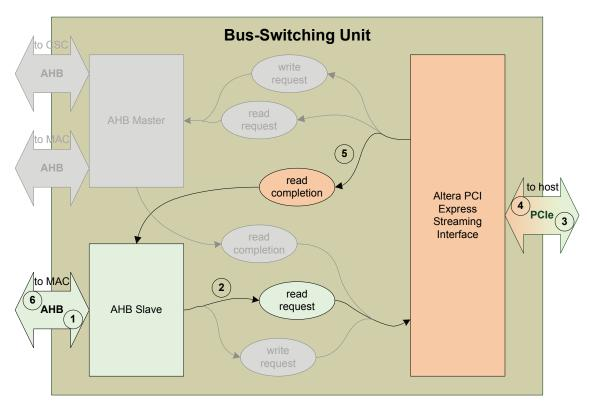
Figure 3.4: Information flow in the bus-switching unit for DMA operation
